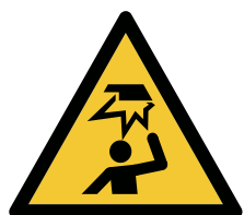
OVERHEAD CRUSH HAZARD
